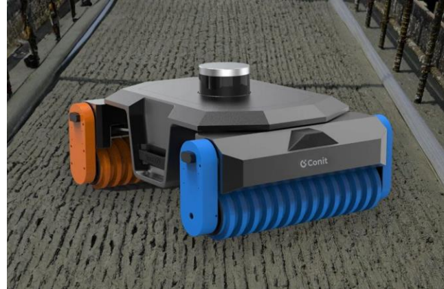
< Robot for creating grooves on wet concrete surfaces CONIT-Runner>
